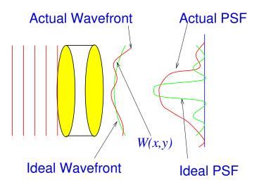
**Define Wavefront Aberration Function** as deviation from ideal parabolic wavefront.
