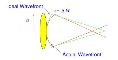
Denote wavefront aberration at edge by  $\Delta W$ , so wavefront aberration is:
