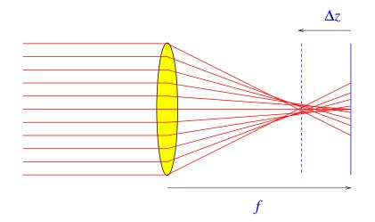
Should be able to "improve" PSF by moving the image plane short of the ideal (paraxial) focus.
