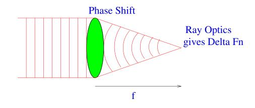
Lens introduces a path length difference, or PHASE SHIFT.
