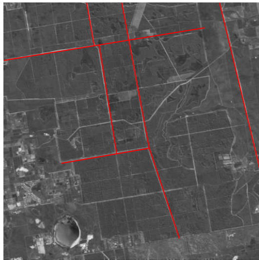
Figure 7: Extraction of linear features, roads in this case, from a satellite image using edge detection followed by analysis using Hough transforms.
