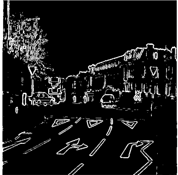
Figure 7: Road scene with two road signs and and binary threshold of edge image.
